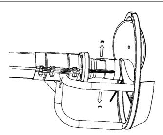
After every use of the BAUER Tractor Turbomix and/or after 5 - 8 operating hours, all greasing points of the mixer must be lubricated with standard grease by means of a grease press (at least 2 full strokes of the grease press at every greasing point).
