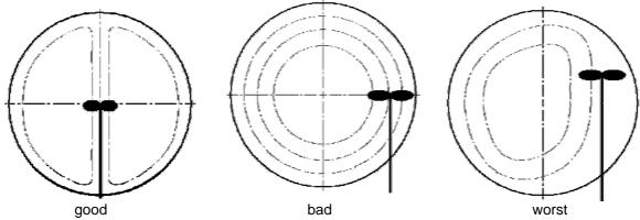
In principle the complete pit content must be made streaming in a way that a complete homogenisation is possible. Make sure that the areas of low current are as small as possible. As can be seen above, in round pits the pit centre is a low current area – when using the mixer as shown on the centre sketch above – where thick matter will conglomerate inevitably.
